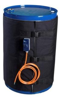
The heating element of the Drum Heaters is stiched into an insulated jacket made from a water resistant, nylon/silicone coated material. Comes complete with quick release buckles for ease of installation and removal. The heating element is shielded with a tinned copper earth braid for safety. All our Drum Heaters are supplied with 3 metres of braided power cable and fitted with a 0 to +90 °C capillary thermostat and 110 volts or 230 volts AC.
