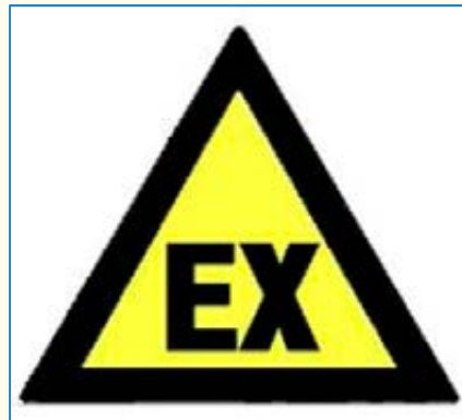
Picture 27: signal that identifies areas with possibility of an explosive atmosphere
