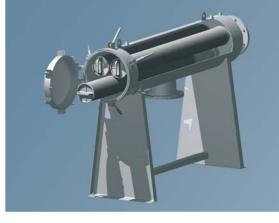
Housings are designed, manufactured, tested, and code stamped in accordance with ATEX Group II, Category 3, T5 and PED 97/23/EC rated Category I. Stainless steel housing external surfaces are glass-bead blasted for a consistent, easy care finish.
