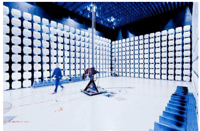
EMC 10-meter anechoic chamber
