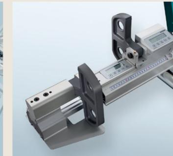
Digital cross-cut fence with continuous support T60A43
