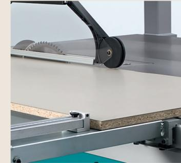
T60A68 second support with T60A55 parallel cutting stop
