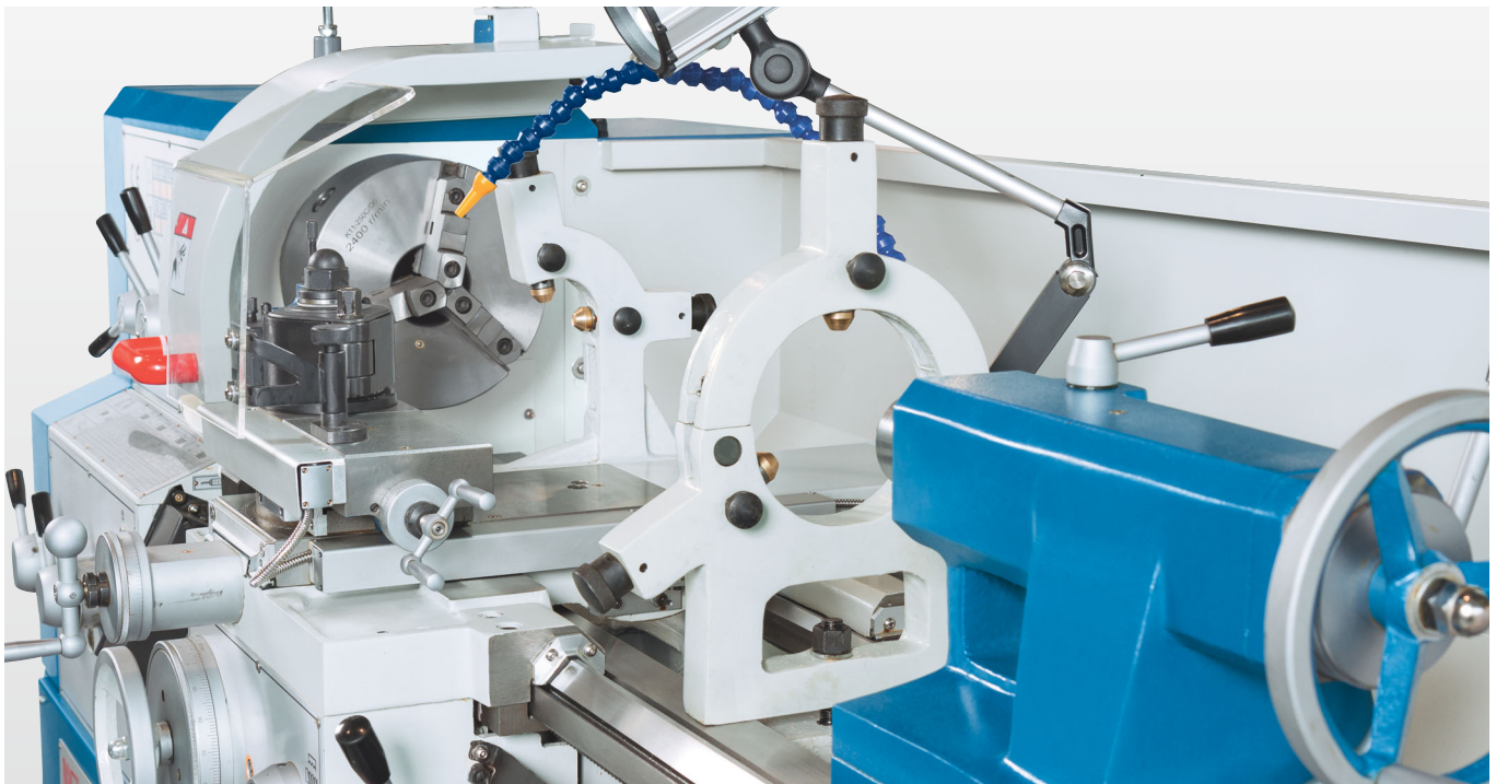
Steady rest and follow rest to support long workpieces
