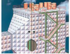
It is essential that filter plates are capable of holding an electric charge in order to guarantee dust attraction. This can only be made possible by selecting the most suitable material.
