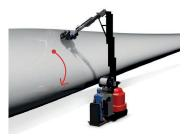
1. Laser sensors on the sanding head detect the top of the blade and start sanding in a downward motion.
