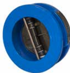
Dual plate wafer check valve for HVAC and water distribution, with lifting ring (for DN200 and above). Suitable for both horizontal and vertical installation. Ductile iron body, stainless steel plates and EPDM seat. Suitable for flanges according to EN 1092-2 PN16 and ANSI class 150, RAL 5015 (blue) epoxy coated.
