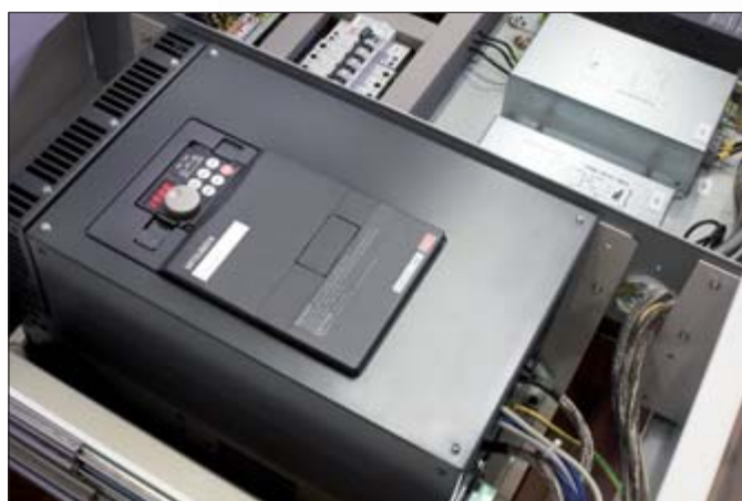
Frekvensomformeren i Hänel Lean-Lift® EcoDrive®
