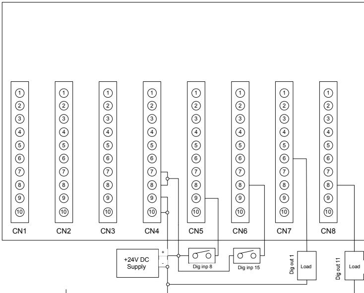
Example: Two digital inputs (switches) and two digital outputs connection.
