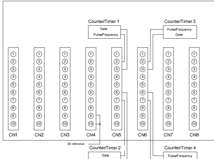
**Example:** Logic connection for four counter/timer measurement. Connection is suitable for counter inputs (pulse and gate) and/or frequency inputs (frequency and gate).
