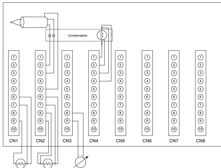
**Example:** Logic connection for various configurations:
