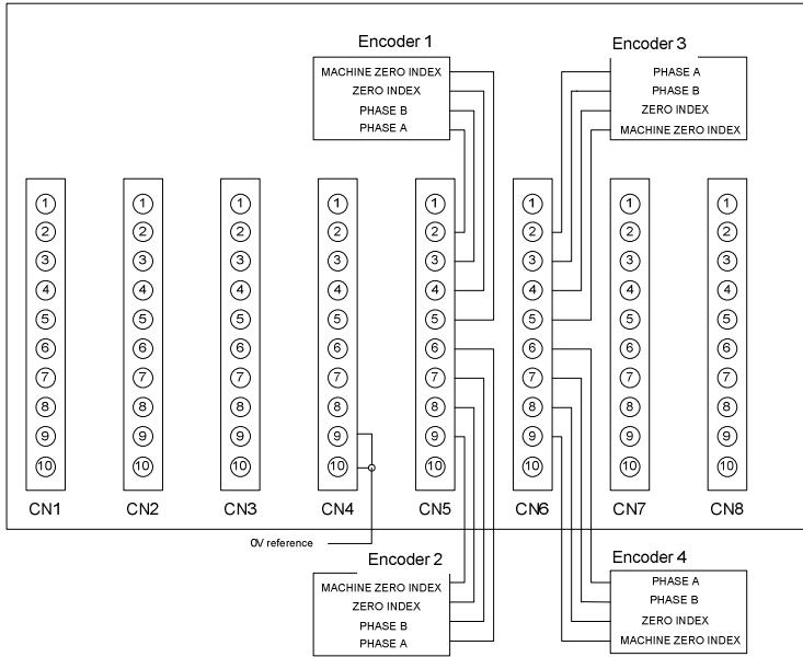
**Example:** Logic connection of four encoder modules. The encoder modules must be 24V powered (connect 0V reference of the encoder to the 0V of PLIO03 digital I/O supply)
