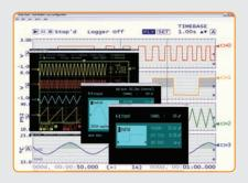
Included **TracerDAQ** software provides set-up capability plus charting and graphing functions. Data can be easily exported into multiple formats.
