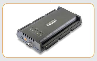
The LGR-5329 is ideal for high-speed data logging. Configuration and data retrieval are made via the SD memory card or USB connection. Built-in control buttons provide the ability to load and save configurations, start data logging, and record triggering events. LEDs provide unit status.
