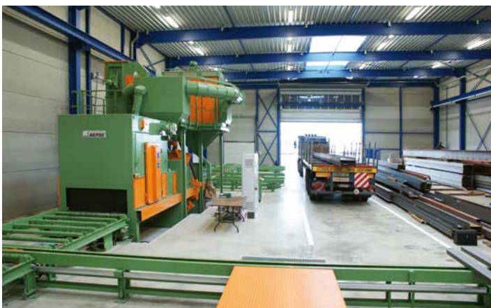
Crossover conveyors connect the roller conveyor shot blast machine with the sawing and drilling machines.
