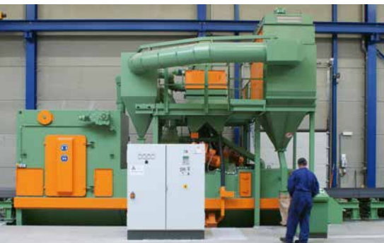
The AGTOS blasting machine with clearly marked maintenance doors
