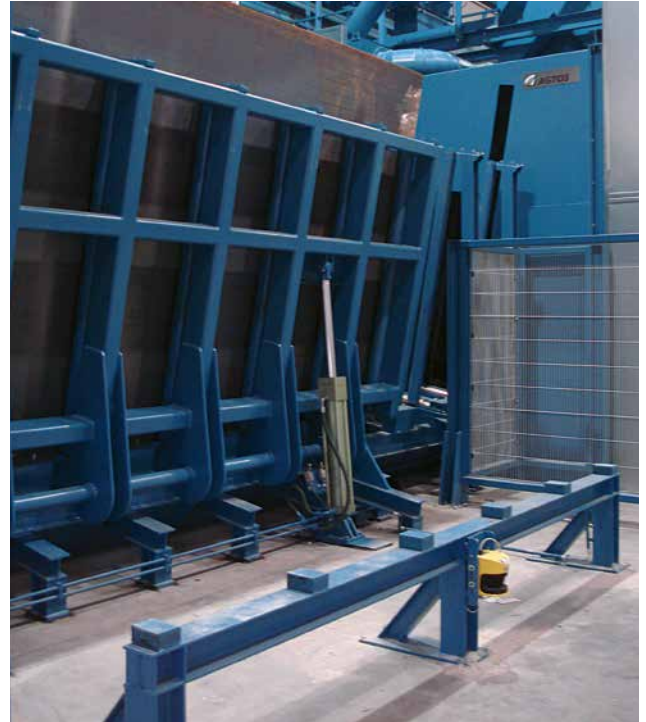
Vertical roller conveyor shot blast machine
