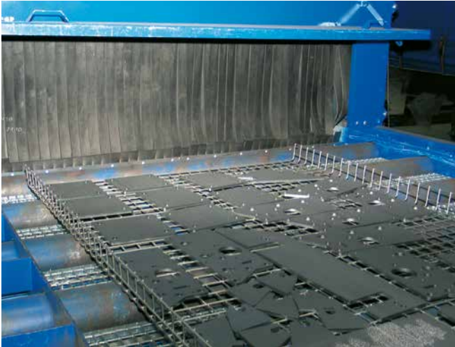
Blasting of flame cut parts in the basket
