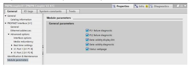
**Data validity display DIA:** The validity of the data is displayed in the bit with the lowest value (Bit 0) of the first input byte of the corresponding PROFINET side:
