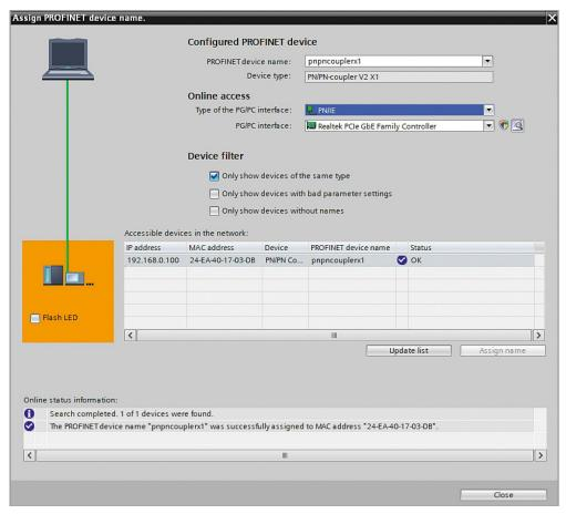
If the PN/PN coupler has received the correct PROFINET name, it is recognized and configured by the PLC. If the configuration is correct, the PROFINET "BF" LED should be off.
