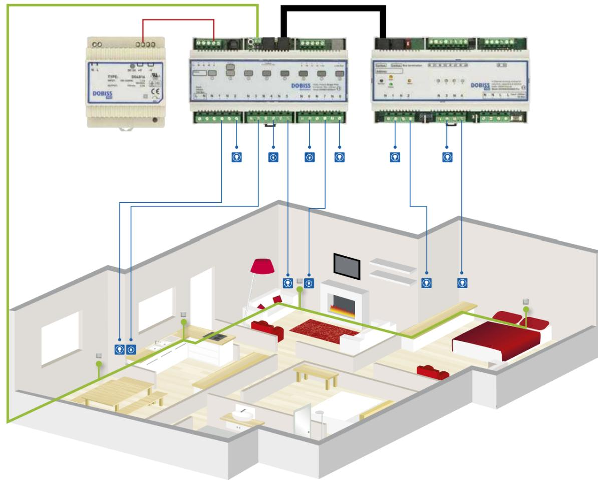
1 twisted pair of the (F)FTP cable is connected from button to button.
