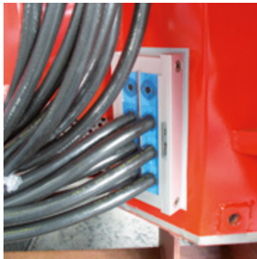
Light railway vehicle: The fire rated Roxtec CF 24 F1 helps ensure passenger safety by preventing the spread of fire into the passenger compartment.
