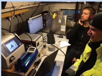
Figures 1 and 2: Experimental setup with measurement equipment inside the van driving next to the selected asphalt paver on a test facility
