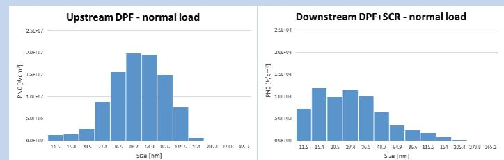
Figures 5 and 6: Average PSD for the asphalt paver, averaged over several measurement cycles of normal operating conditions and measured with NanoScan SMPS. PSD are shown in the full measuring range of 10-420 nm. Note that the scales on the y-axes differ by a factor of 1,000 on the two figures
