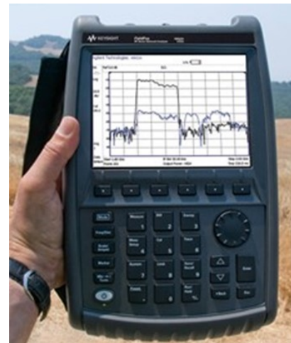
Read measurements in direct sunlight with the transfective display
