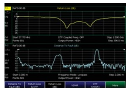
View return loss and DTF simultaneously
