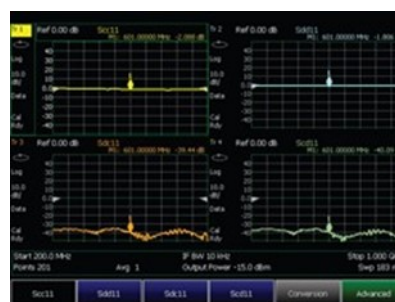
Characterized common and differential mode reflections with mixed-mode S-parameter measurements
