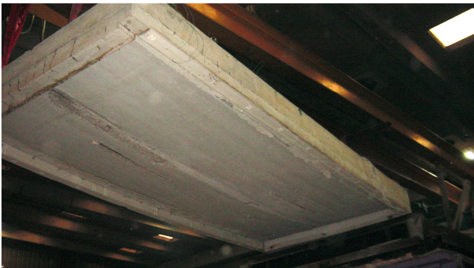
Figure 3. Test H138 in [2]. Hollow-core slab after 25 min. Photo K. Hertz.
