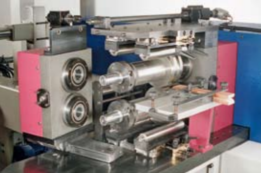
Standardmässig ausschwenkbares Schiebelager und motorisch verstellbare Messerwellen Equipped as standard with pivotable sliding bearing and motor driven cutter shaft adjustment
