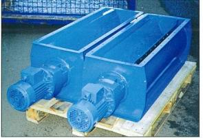
The Aagaard rotary valve is designed to control the flow of waste, such as wood shavings, dust, granulate, corn and a wide range of other materials from collection, transport systems and silos.
