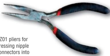
SZ01 pliers for pressing nipple connectors into hollow round belts.
