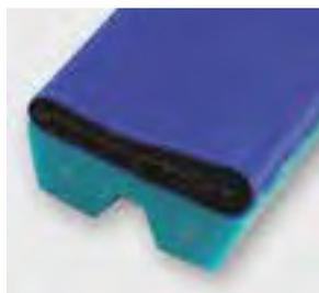
PU85A Twin-V-belt (30x8 mm) with reinforcement Polyester and neoprene coating. Especially for PET bottle transport / guide.
