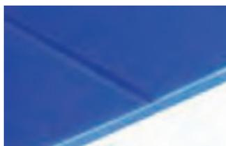
Butt welding with paddle welding tool
