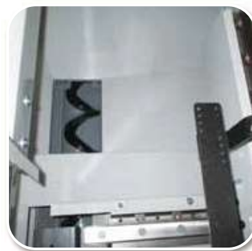
Drainage outlet & Chip auger
