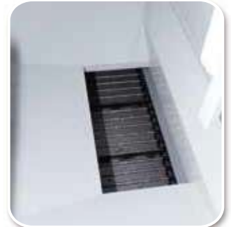
Drainage outlet & Chip conveyor
