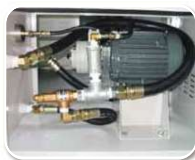
CTS system with high pressure 20bar pump
