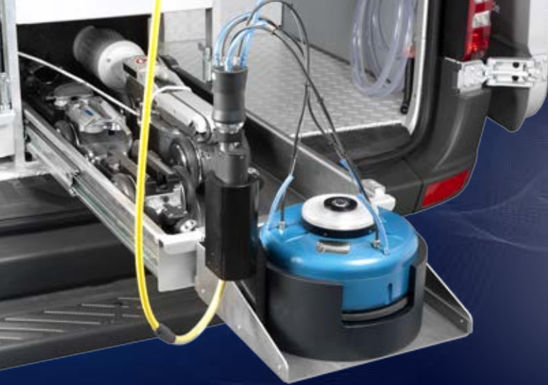
At the top: PANORAMO-SI-shelf for insertion into the camera drawer.
