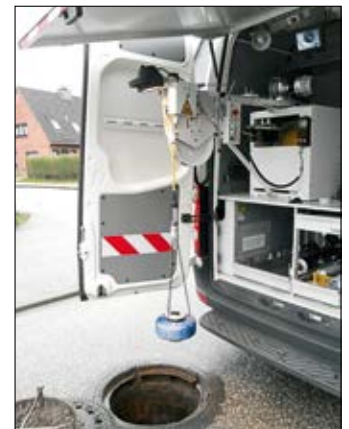
PANORAMO SI as pallet installation kit for the VW T5 (autarkic compact module) and as extension to an inspection system
