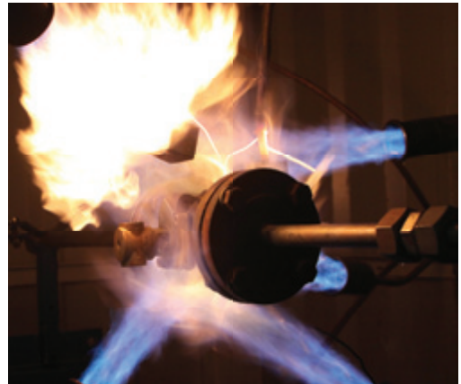
2" 73Z valve in a fire test
