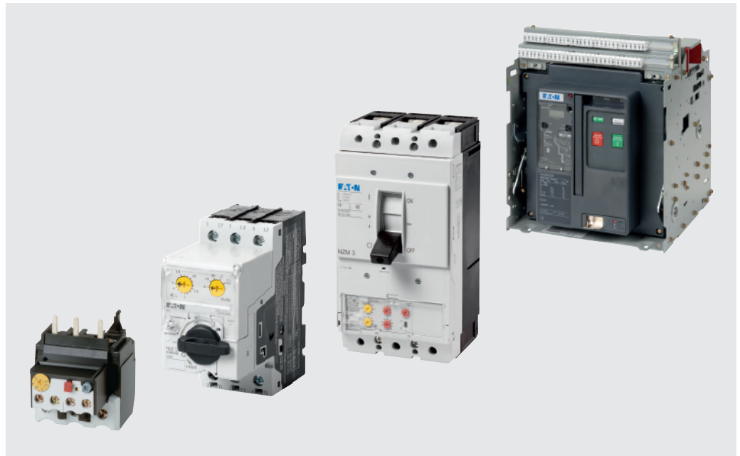
Figure 2: The four frame sizes of the Eaton NZM compact circuit-breakers. Frame sizes NZM 1, NZM 2 and NZM 3 feature a thermo mechanical and electromechanical release. The frame sizes NZM 2, NZM 3 alternatively feature electronic releases as with the NZM 4 and the open circuit-breaker IZM as shown on the left.
