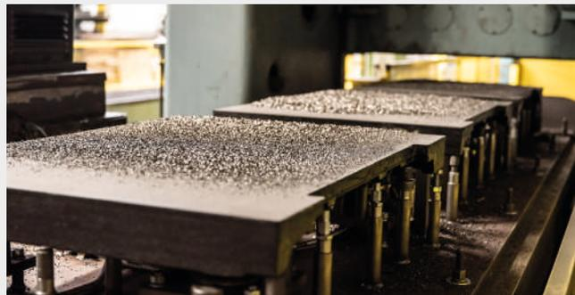
Surface scraping of cast iron table
