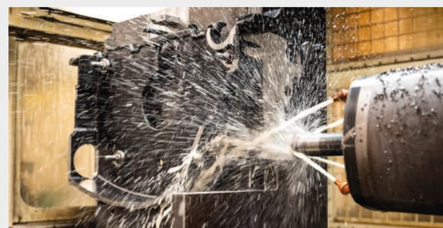
CNC Machining of cast iron saw aggregate
