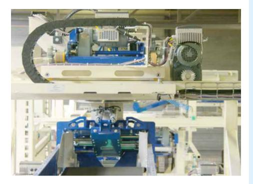
Decentralised drive units consisting of a gear unit, motor and electronics replace centralised servo technology and enable highest dynamic levels for palletising.
