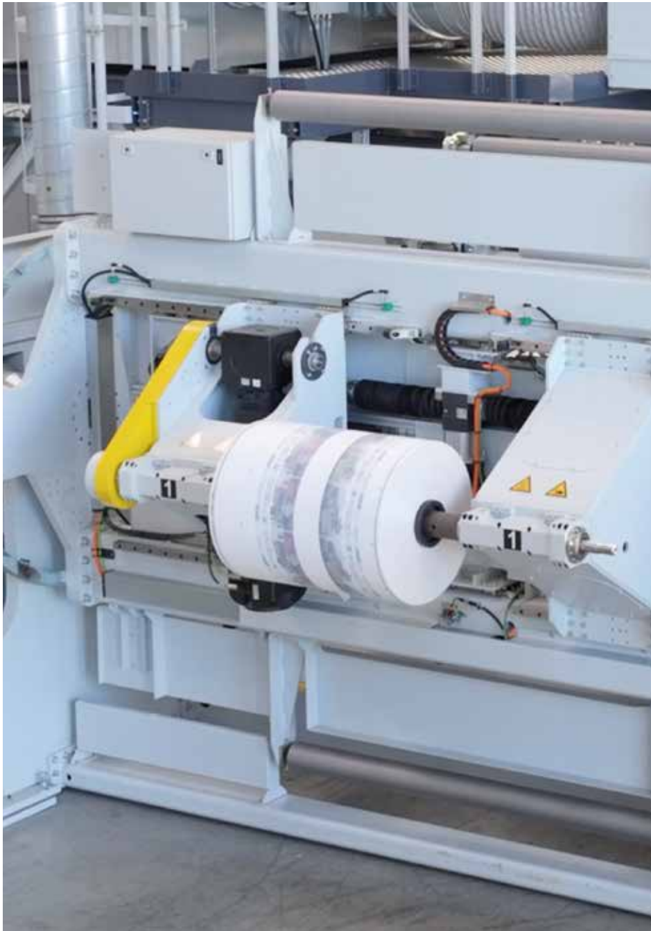
UW 1500 WS – shafted winding
