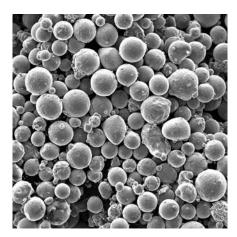
Manufacturing technology and continuous process control ensure spherical powder with optimal properties for 3D printing.
