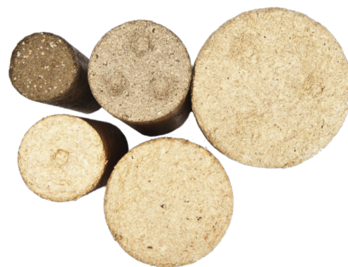
Briquettes with diameters 50, 60, 75, 90 and 120 mm
