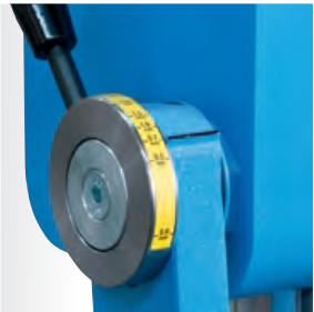
Adjust clamping pressure with a lever
