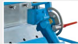
Adjust bending angle with scale and lever
