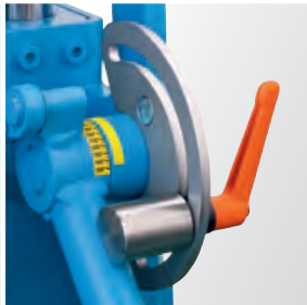
Adjust bending angle with scale and lever
