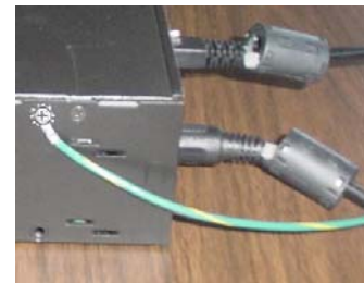
This partial view of a data acquisition device shows its connection to the ground-line. It also shows two ferrite collars, the foremost of which is clamped to the power cable. The background collar is clamped onto the Ethernet cable.
