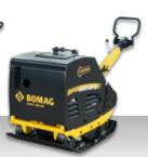
BPR 100/80 D Operating weight: 710 kg Centrifugal force: 100 kN Working width: 800 mm
