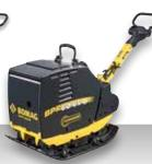
BPR 60/65 D Operating weight: 460 kg Centrifugal force: 60 kN Working width: 650 mm
