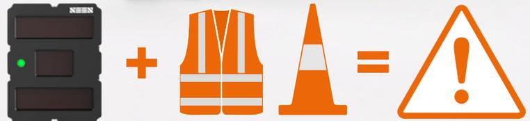
IRIS 860 sensors make pedestrian detection easy by detecting the reflective tape on high-vis safety vests and markers. If a pedestrian enters the critical risk zone they and the driver receive an audible alert.
