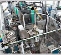
Automated overmoulding: robots can also be used as a reliable way to feed in flexible inserts.
