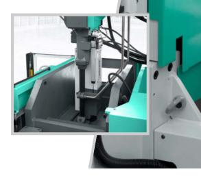
Simple changeover: central connection of all cylinder module supply units and screw quick-connect coupling.
