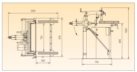
Dowel hole boring machine D-23 is purposed for vertical and horizontal drilling of surface and other furniture elements. This machines is very suitable for quick exchange of production program.
