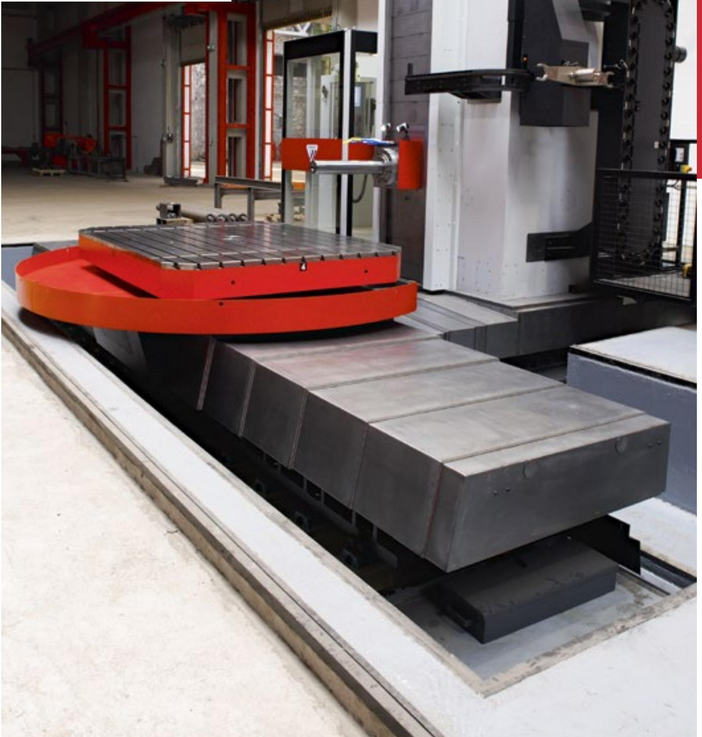
Parameters: X=5 000 mm (196.85") | Y=2 500 mm (98.43") | Z=2 000 (78.74"), W=730 (28.74") | Rotary Table = 1 800 x 2 600 (70.87x102.36")
