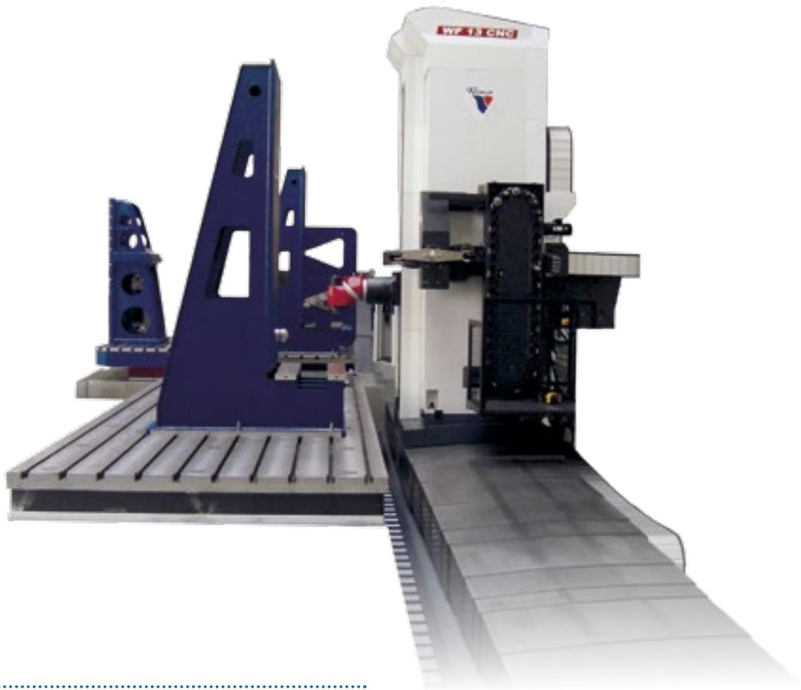
A Floor type horizontal boring mill WF type is designed for precise and highly efficient coordinate boring, drilling, milling, and cutting of threads of big and heavy work pieces up from cast iron, cast steel and steel. The machine can be equipped with floor plates and/or rotary table(s) according to machining requirements. As with all Fermat Boring Mills a wide range of accessories can be added that considerably enhance the machine's versatility.
