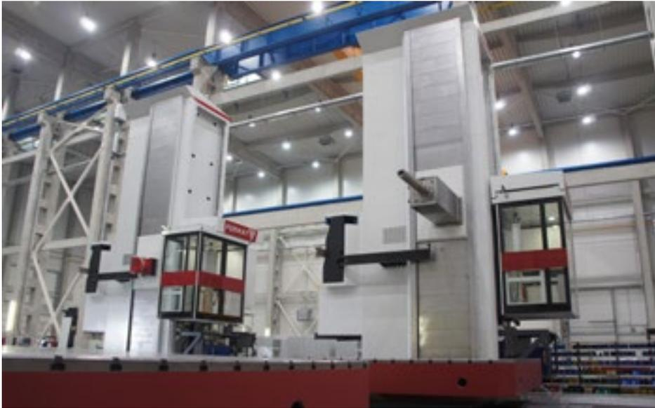
Heavy duty execution of floor type boring mill with ram stroke 1 500 mm (59.06"), 1 000 mm (39.37") spindle stroke with 160 mm (6.30") spindle diameter represents the newest technology and concept of floor-type horizontal boring mills that are currently on the global marketplace. The powerful closed designed headstock consists of a movable slide ram (Z-Axis) and a movable live spindle (W-Axis).
