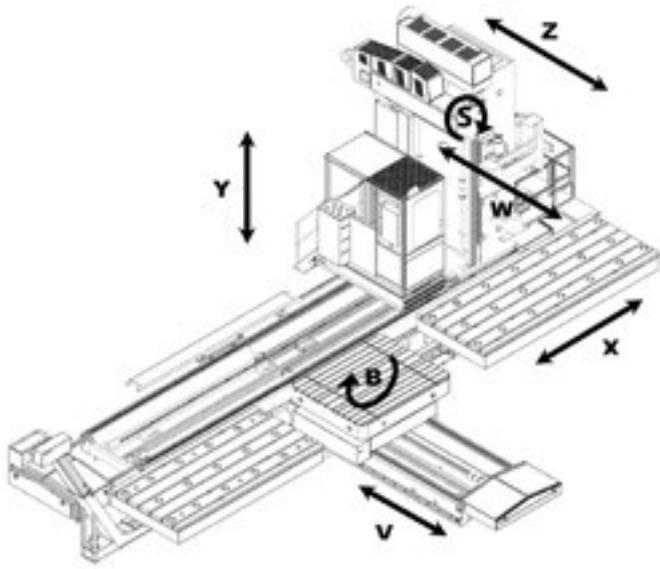
Horizontal Boring Machines WRF are the biggest representatives of FERMAT boring mill production. They are used mainly for precise and powerful machining of big and heavy work pieces from iron, cast steel and steel. Our machines are usually intended for machining of large energy parts, crane or ship parts, oil and gas equipment and similar applications.
