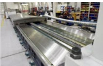
X-Axis Hydrostatic guideways
