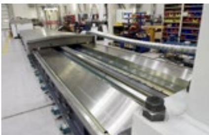
X-Axis Hydrostatic guideways
