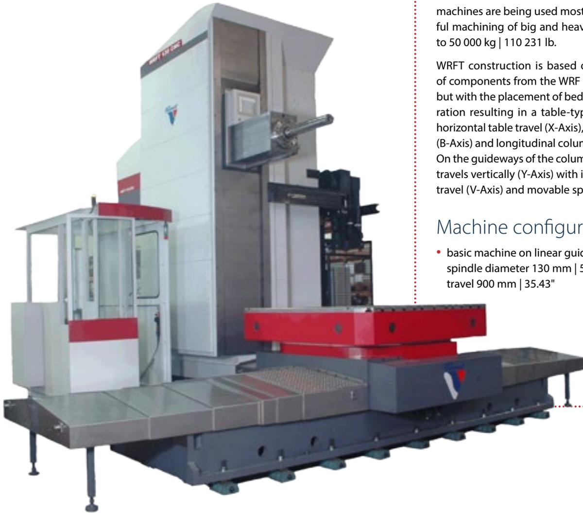
The horizontal milling and boring machines WRFT represent the newest technology and concept of large table type horizontal borers with ram travel and movable spindle. WRFT machines are being used mostly during powerful machining of big and heavy workpieces up to 50 000 kg | 110 231 lb.
