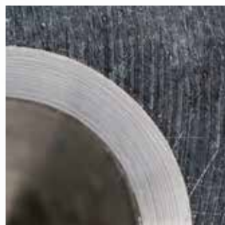
countersinking with V-NX countersink
