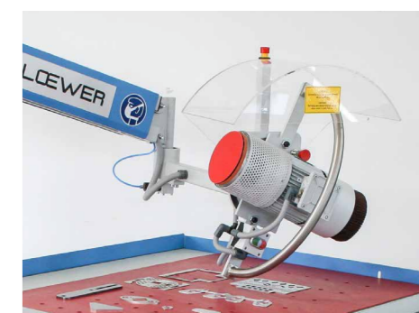
180° tiltable head for quick access to deburring and edge rounding tools
