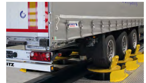
Test distance: 1,000,000 km. The results on the hydropulsers help to optimise the entire vehicle.
