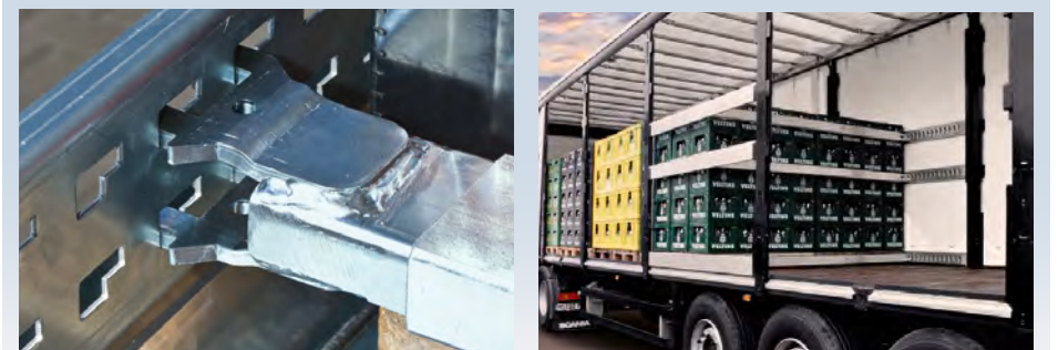
The cross beams can be positioned precisely using the flexible load securing system with a perforated grid in the steel support slats. They are inserted with two simple motions.
