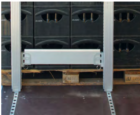
Short support slats can also be used in between the load securing bars for securing the load in the beverage industry.
