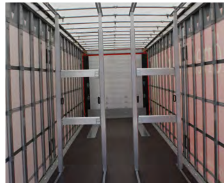
Four full-length perforated grid rails provide rapid securing of interlocking partial loads with locking bars.
