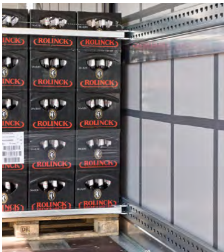
Transverse beams at the front and rear of the freight secure partial loads against sliding longitudinally.
