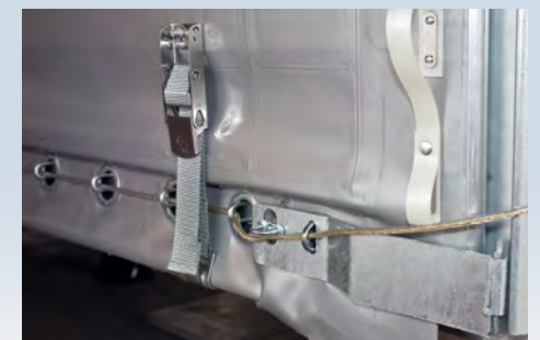
Covering plates on the front and rear tarpaulin tensioners along with crimps on the outer frame ensure that the cargo is sealed for customs. All of the securing elements are connected with the full-length customs cable and the lead sealed.
