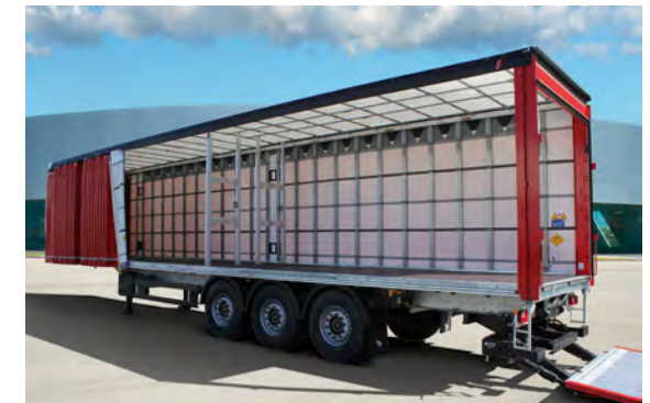
Robust aluminium, fixed-design tail lift with pendulum tailgate. Roll-off prevention for 2 roll containers and the separate side battery ensures safe work when loading and unloading.
