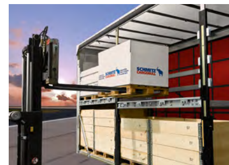
Two cross beams are provided for one pallet row in a grid of approx. 1,200 mm.
