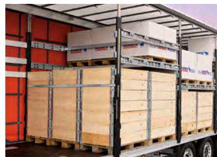
Cross beams between the stanchions or side support beams allow the second level of freight to be securely loaded.
