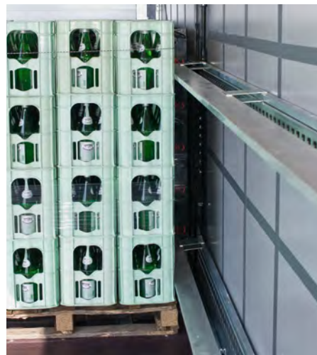
Spacing slats are folded so that they interlock along the sides for the transportation of well pallets.
