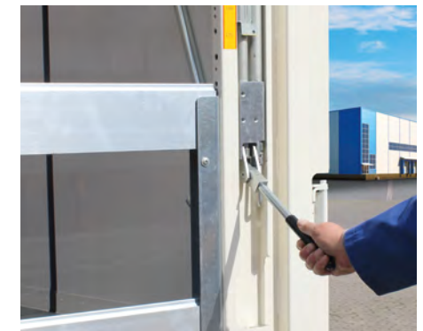
The mechanical lifting equipment in the corner stanchions enables the roof on MEGA trailers to be raised manually.
