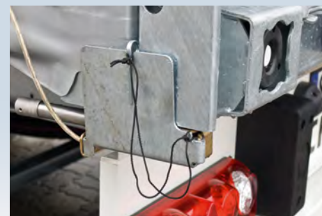
Covering plates on the front and rear tarpaulin tensioners along with crimps on the outer frame ensure that the cargo is sealed for customs. All of the securing elements are connected with the full-length customs cable and the lead sealed.
