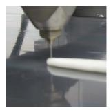
Further you achieve a glue line or spot which is larger, more filling, which is a great advantage by applications, where the glue is used for sealing or where the involved materials are flexible, i.e. for textile gluing where it normally is difficult to obtain a good contact surface.
