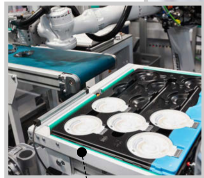
Film insert moulding: excellent repro- ducibility with servo-electric drives.
