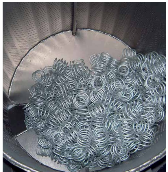
Drum shot blast machine for the hardening of coil springs
