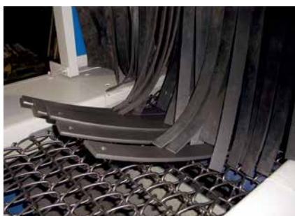
Outlet of a wire mesh conveyor shot blast machine for the hardening of leaf springs
