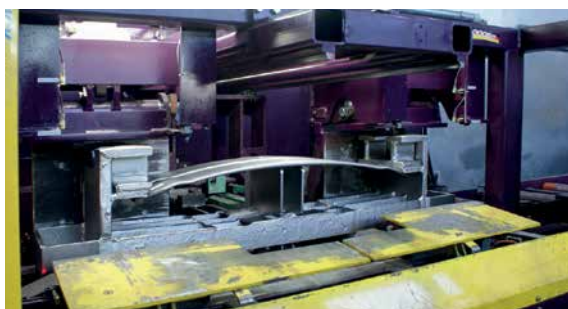
Pre-stressing machine for leaf springs before processing in a roller conveyor shot blast machine
