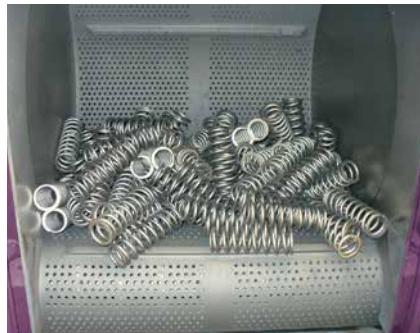
Rubber belt tumble shot blast machine for hardening coil springs
