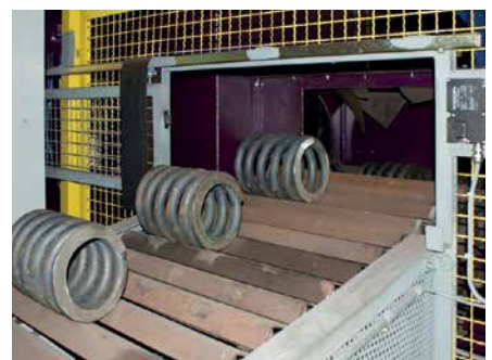
Inlet and outlet of a walking beam shot blast machine for the cleaning of coil springs
