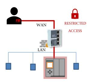
For purposes of segmentation, the REX routers are equipped with a WAN interface for the factory network and a LAN interface for the machine network.
