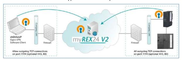
Likewise, integration into local firewalls is simplified with the VPN portal. Local firewalls are connected to the WAN network of the router. Access from the Internet to the REX router is usually prohibited. Outgoing connections are often allowed or can be easily and securely realized. The router then in this way "dials" into its account on the central VPN server.
