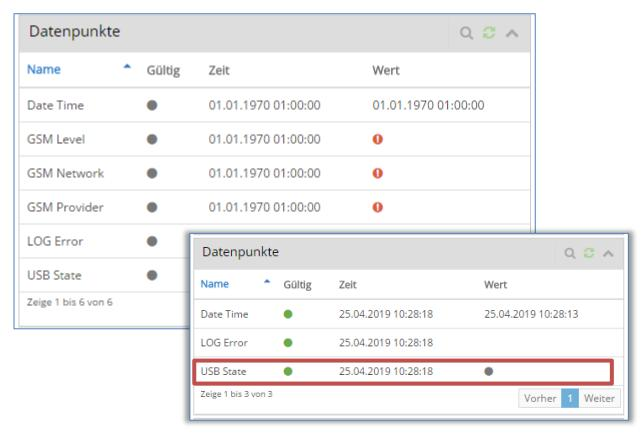
Various data points are available depending upon the version of the device. When the USB socket is not required for the application, it is recommended that this be deactivated. Depending upon the configuration of the router, the USB interface can be addressable in a network via the LAN.
