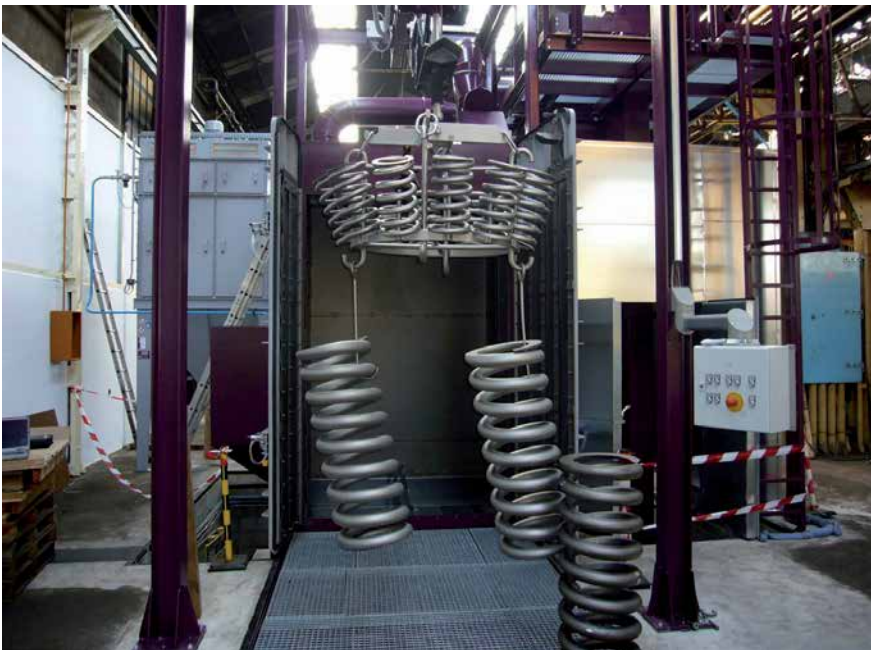
Overhead rail shot blast machine with baseplate and blasting abrasive recirculation for the treatment of springs
