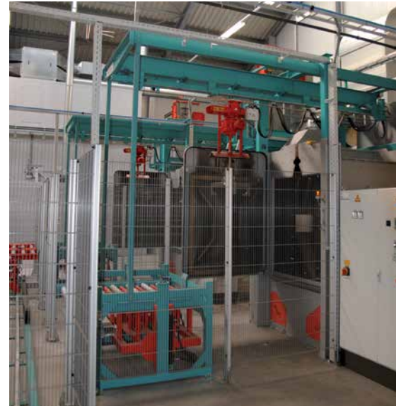
Overhead rail shot blast machine for connecting components in a production line
