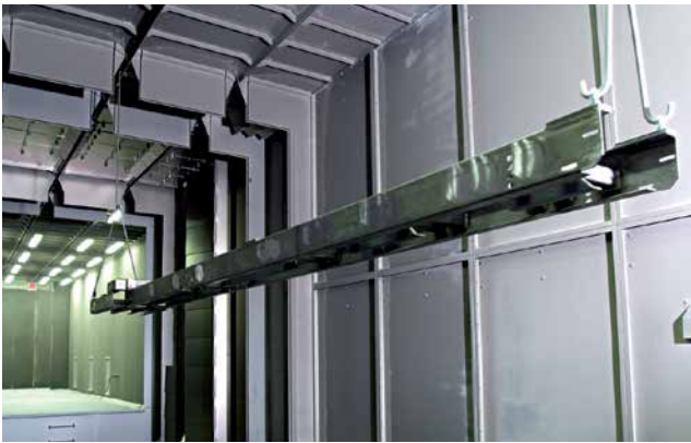
Continuous overhead rail shot blast machine for welded components with manual re-blasting and blowing chamber
