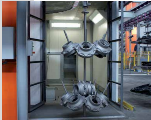
Cast parts exiting the manual blowing chamber of a dual-chamber overhead rail shot blast machine
