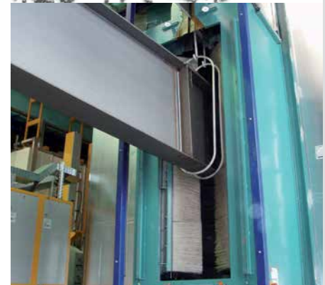
A steel girder after blasting in a continuous overhead rail shot blast machine
