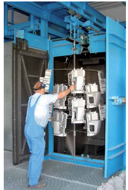
Overhead rail shot blast machine in a foundry with magnetic separator and blasting abrasive recirculation upstream of the machine
