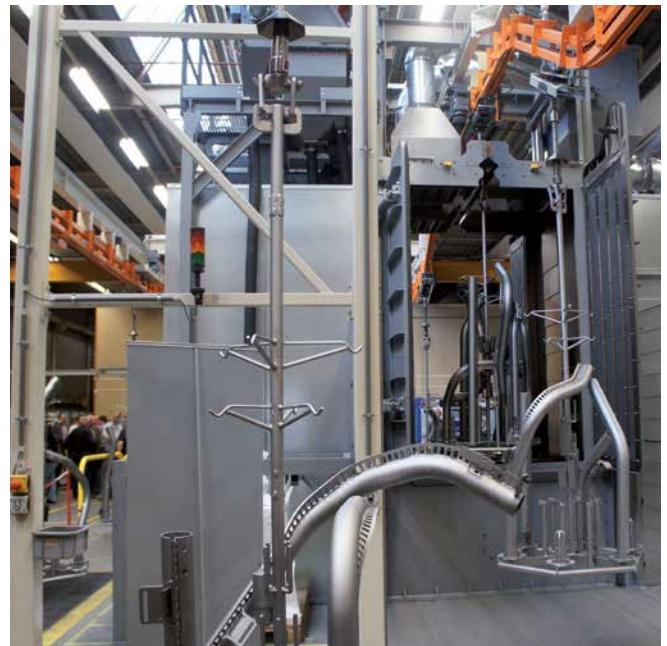
Continuous overhead rail shot blast machine for welded components with turbines on one side
