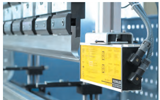
Ce Laser Safety System
