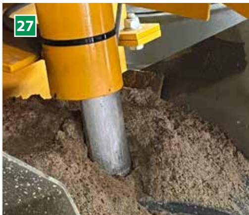
27 Moisture sensor for hopper (optional) Sensor for measuring moisture in the dosed sand prior to entering the mixer.
