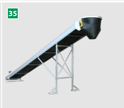
35 Belt conveyors (optional) Belt conveyors with belt widths of 0.8 m or 1.0 m and lengths of 8m - 14 m. Available with height-adjustable legs or hydraulic system for automated operation. All conveyors are equipped with a drum motors, integrated gearboxes, inlet boxes, dispenser funnels, and lifting hooks for easy transportation.
