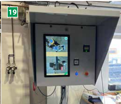
19 Payment terminal for Fibo Collect (optional) Terminal with 21" touch screen including software for your Fibo Collect plant. The terminal is equipped with a barcode reader and a thermal printer. Requires Fibo Link
