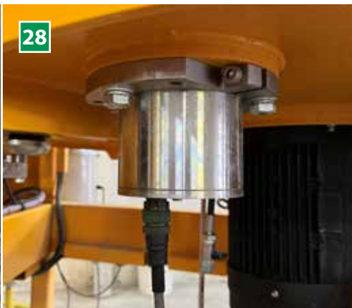
28 Moisture sensor for the mixer (optional) Moisture sensor mounted in the mixer to indicate batch moisture level.
