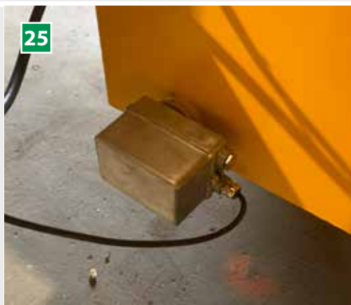
25 Water heater (optional) Electric heating in the water tank for frost protection. Complete with thermostat and switch. The heater is usually connected to the control cabinet for automatic operation and frost protection. Power 4 kW. Voltage 3 x 400 volts.
