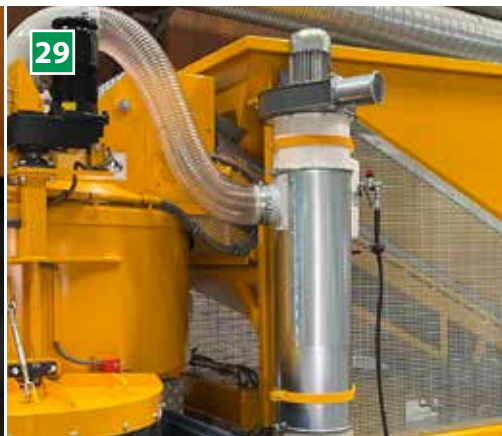
29 Dust filter for the mixer (optional) Filter to reduce cement dust in the environment during the dosing process.
