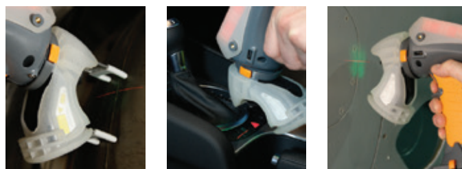
Split laser line adjustment, small laser line adjustment, long laser line.
