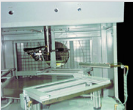
Standard ion luftkniv renser metalrammer inden pulverlakering.
